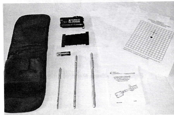
Figure C-1 Standard Laser Borelight Kit
